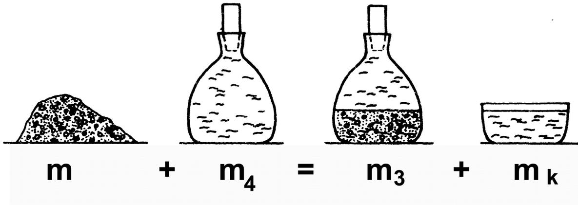
where  $m_k$  is mass of liquid, volume of which was pushed up by volume of the solid material
